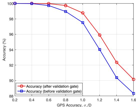
Fig. 6. TMA vs. Ratio of standard deviation of GPS error to the desired separation.
