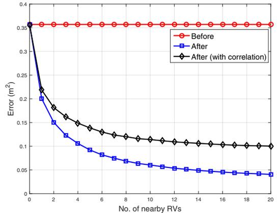
Fig. 4. MSE (m<sup>2</sup>) vs. Number of nearby DSRC equipped RVs.
