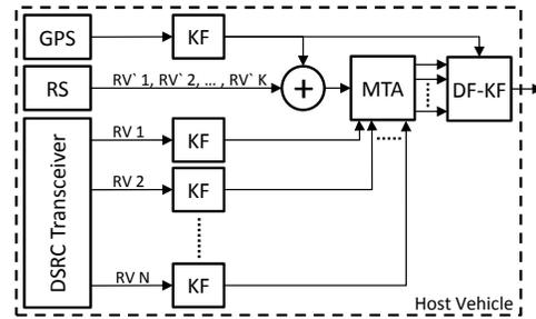
Fig. 3. Positioning improvement algorithm design.
