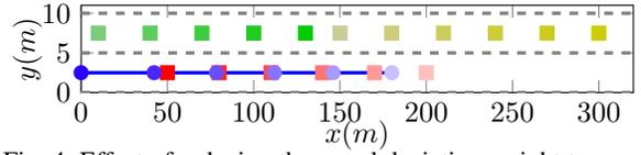
Fig. 4: Effect of reducing the speed deviation weight to  $q_1 = 0.5$  in the overtaking scenario. The position of the ego vehicle is shown as blue dots, and rectangles with different colors mark the positions of surrounding vehicles. Time dimension is color-coded, with lighter colors corresponding to instants further away in time.
